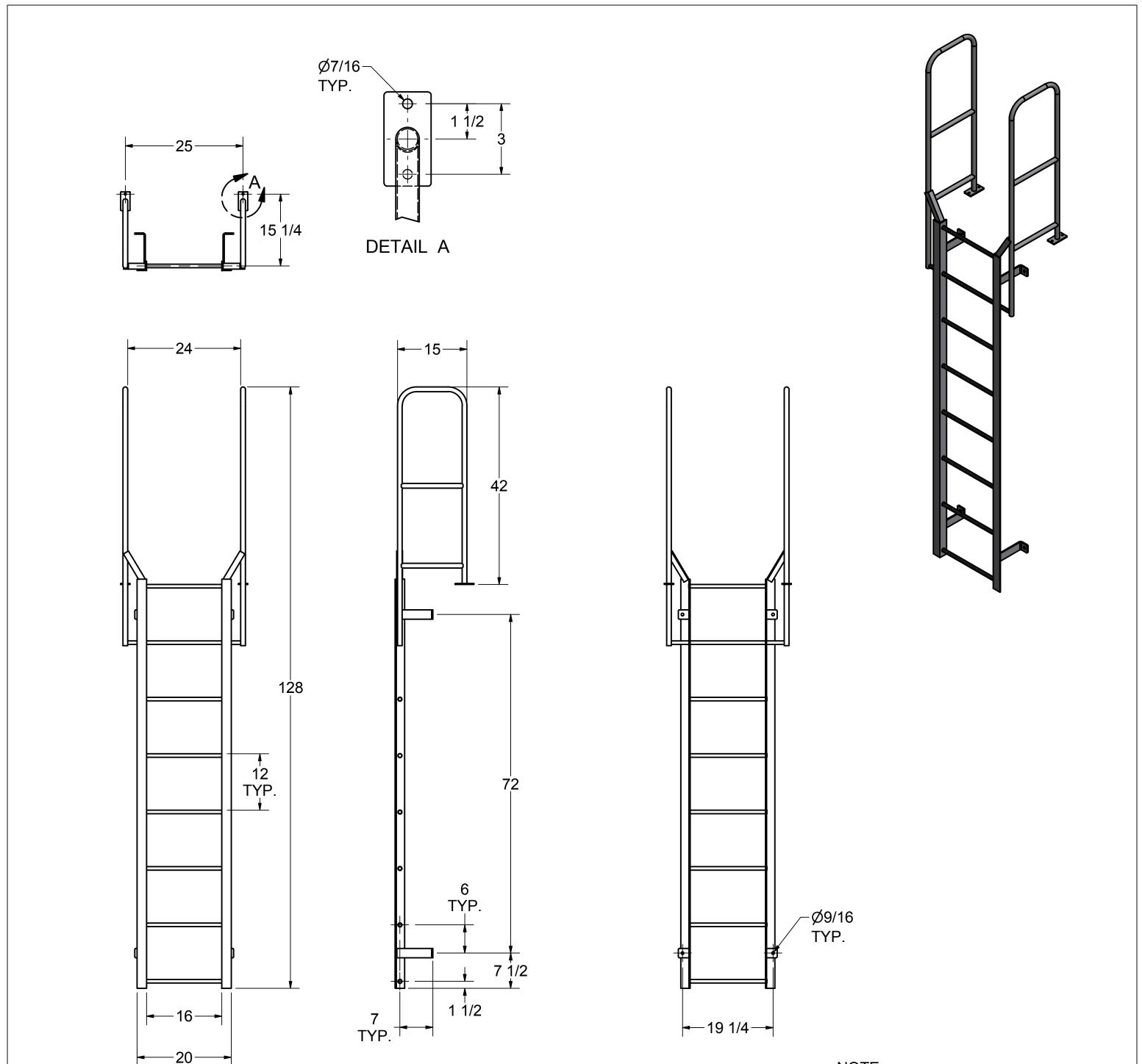
NOTE: STANDOFF BRACKET LOCATIONS ARE ± 1". DO NOT PREDRILL HOLES IN THE STRUCTURE. HOLES SHOULD BE MATCH DRILLED TO INSURE PROPER ALIGNMENT
