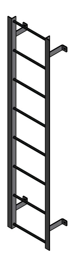
NOTE: STANDOFF BRACKET LOCATIONS ARE ± 1". DO NOT PREDRILL HOLES IN THE STRUCTURE. HOLES SHOULD BE MATCH DRILLED TO INSURE PROPER ALIGNMENT
