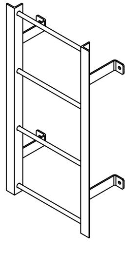
NOTE: STANDOFF BRACKET LOCATIONS ARE ± 1". DO NOT PREDRILL HOLES IN THE STRUCTURE. HOLES SHOULD BE MATCH DRILLED TO INSURE PROPER ALIGNMENT
