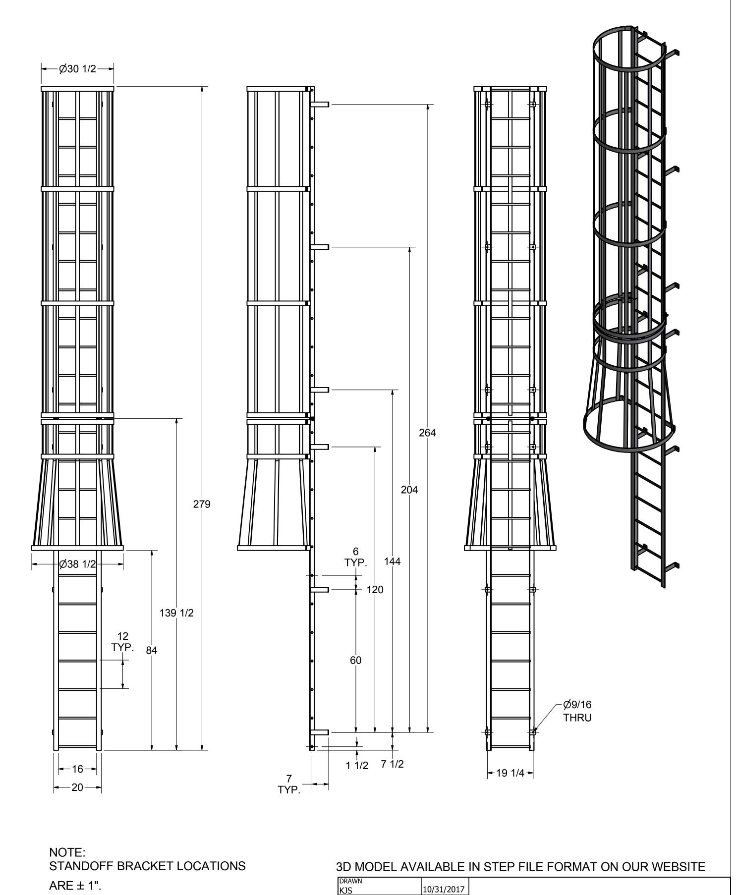
DO NOT PREDRILL HOLES IN THE STRUCTURE.
