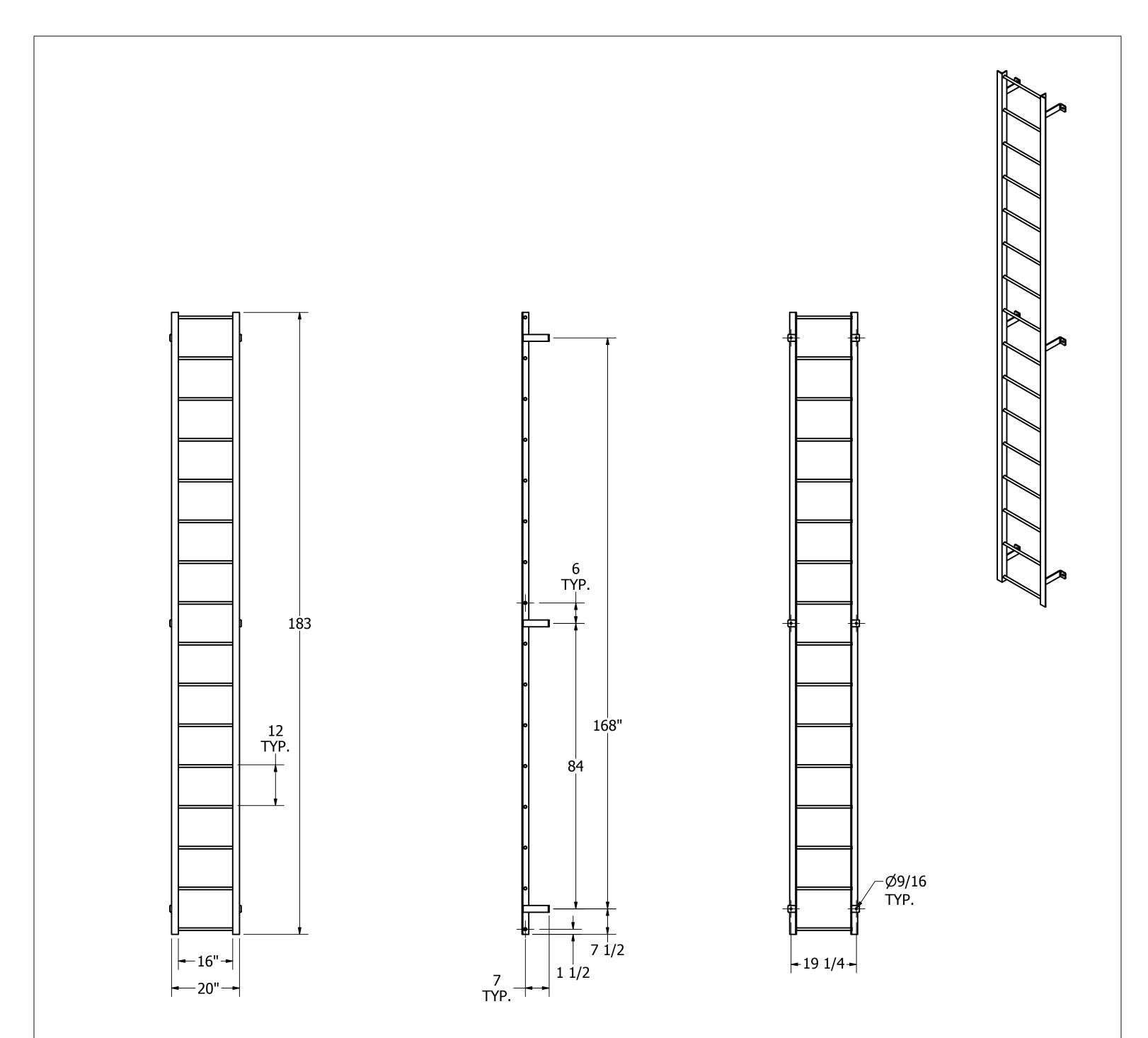
NOTE: STANDOFF BRACKET LOCATIONS ARE ± 1". DO NOT PREDRILL HOLES IN THE STRUCTURE. HOLES SHOULD BE MATCH DRILLED TO INSURE PROPER ALIGNMENT
