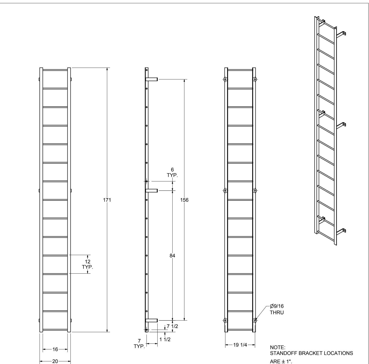
ARE ± 1". DO NOT PREDRILL HOLES IN THE STRUCTURE. HOLES SHOULD BE MATCH DRILLED
